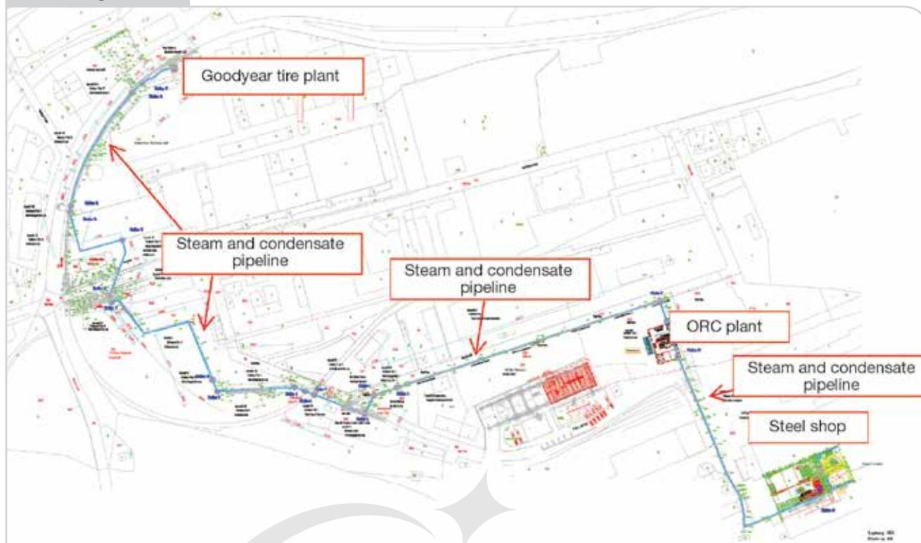
Steam and condensate pipelines overall layout at Riesa.
