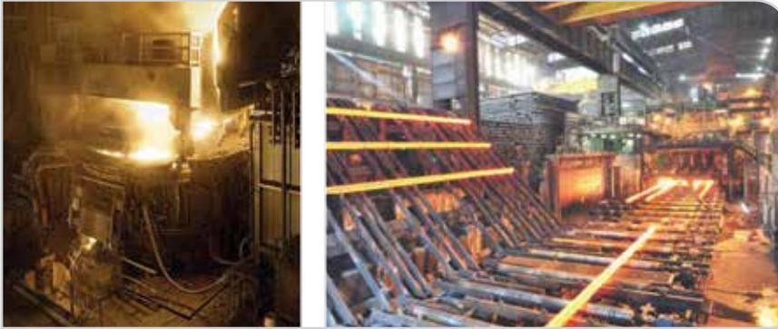
EAF (left) and continuous casting machine (right) at ESF, Riesa.
