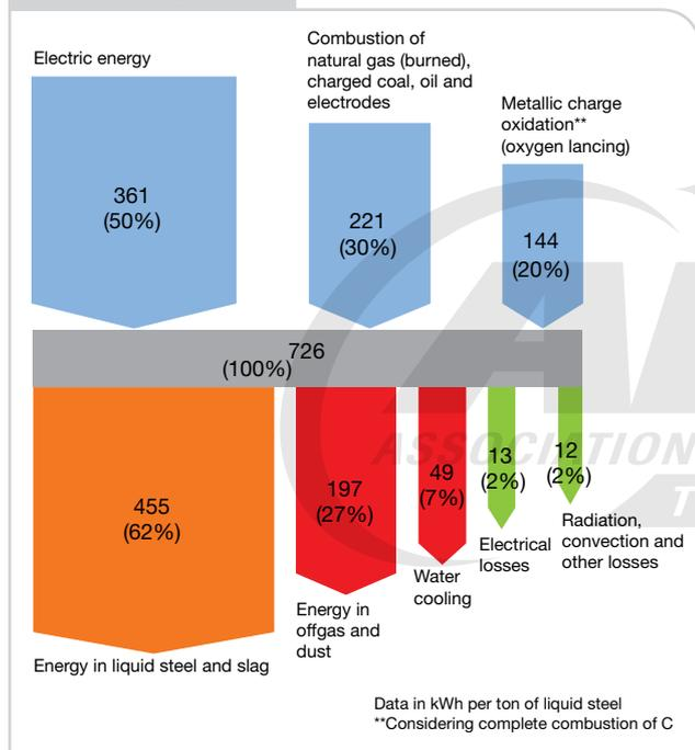
Typical energy balance for top-charged scrap-based EAF (Tenova).
