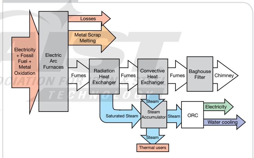
Heat recovery system with ORC technology from exhaust gas of EAF, as applied in Riesa.
