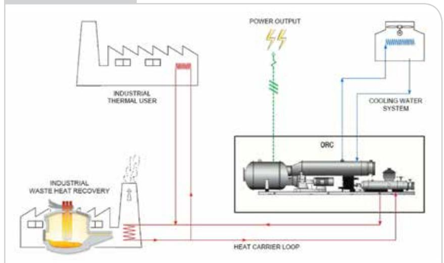
Simplified cogeneration waste heat recovery scheme, as applied in Riesa.
