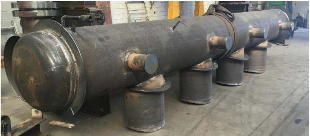
**Figure 10 Regenerator outlet shell**
