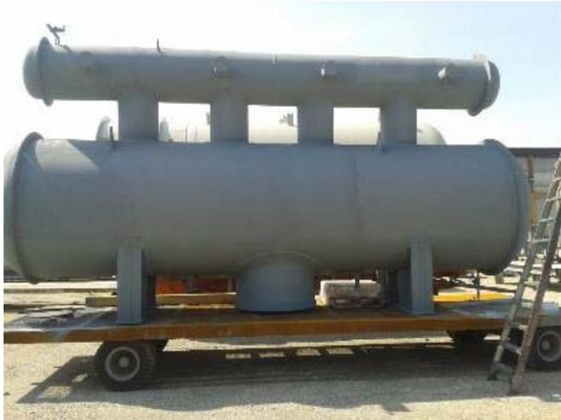
**Figure 11 Completed regenerator**
