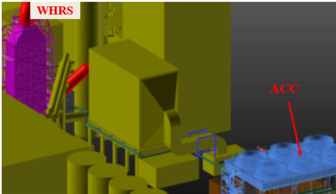
Figure 5 Overall view of main ORC components
