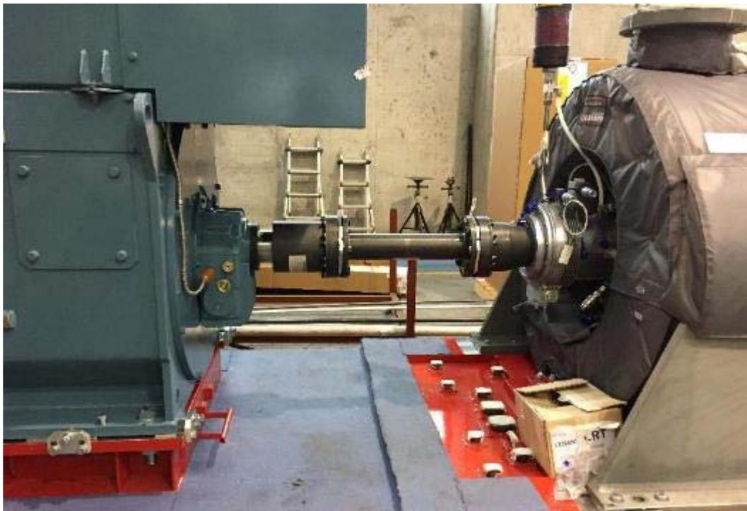
**Figure 14 Turbine coupled to the generator**
