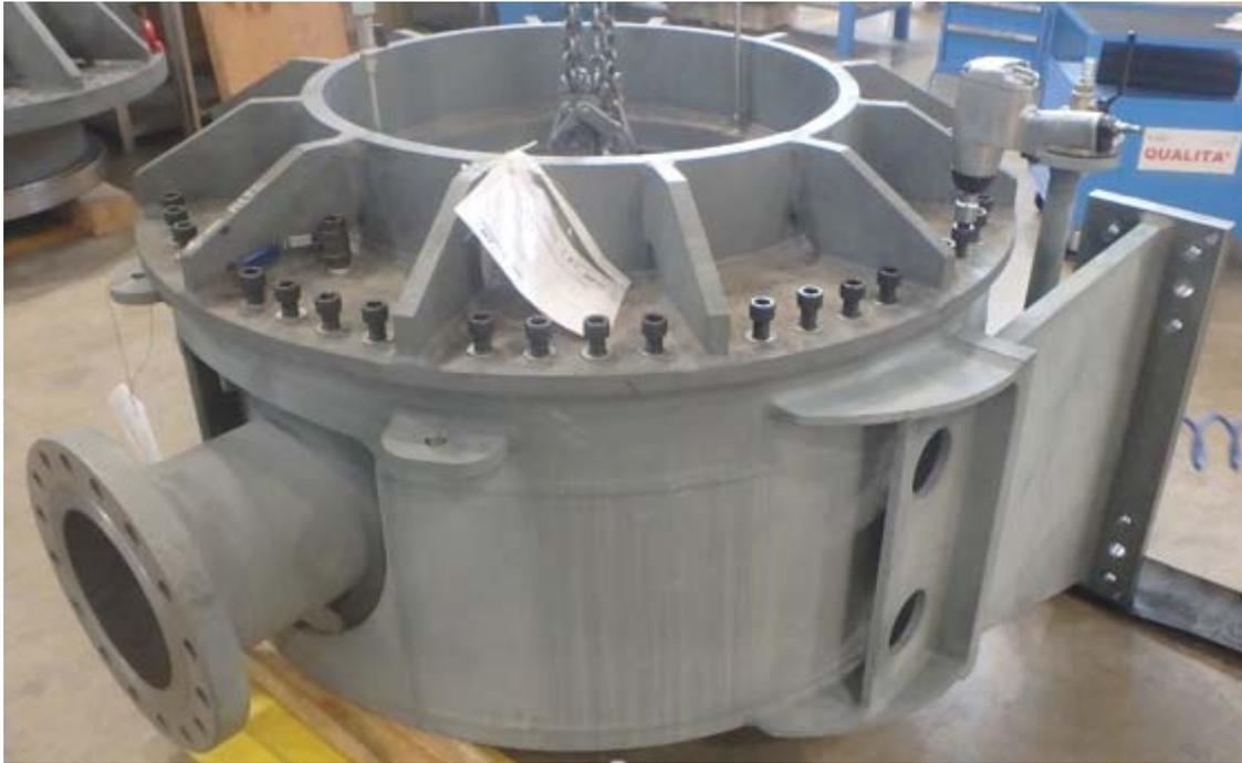
**Figure 13 Turbine casing with tools for pressure test**
