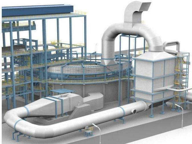
Fig. 1: Waste heat recovery at Sinter Cooler
