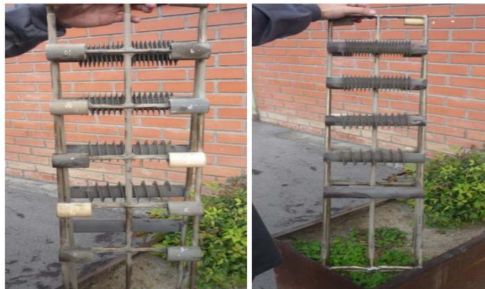
**Figura 3: Metallic frame containing samples obtained by the combination of 3 steels and 4 coating materials recovered from the interior of the chimney in SIDENOR's plant after the 4 month long test.**
