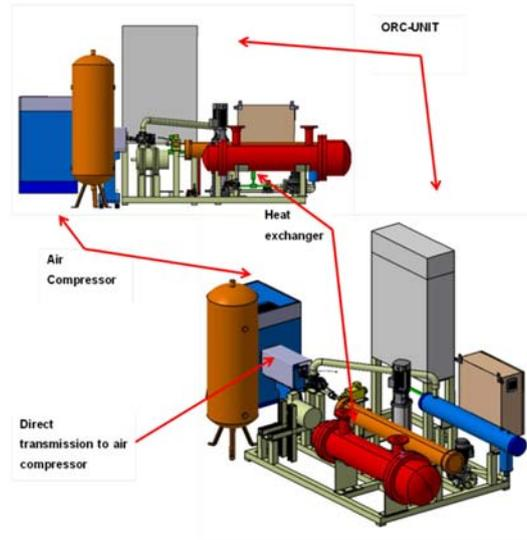
**Figure 3: Layout of the pilot demonstrator designed to validate the concept for the generation of compressed air with the use of combustion gases.**
