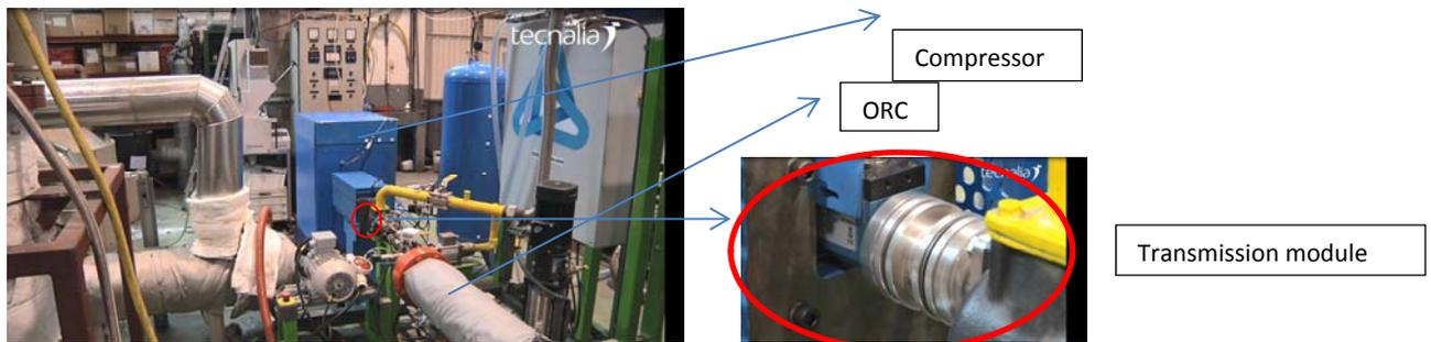
**Figure 1: Pilot installation for the generation of compressed air from hot gases. Detail of de transmission module developed in the project.**
